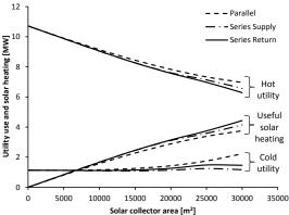
Figure 3: Composite curves for Solar-HRL hybrid system with series solar collectors.
