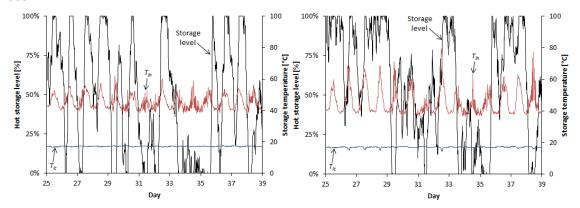
Figure 5: Hot storage tank levels and hot and cold storage tank temperatures for the Solar-HRL hybrid system with parallel solar (a, left) and return series solar (b, right), with 15,000 m<sup>2</sup> solar collector area and 500m<sup>3</sup> tank volume
