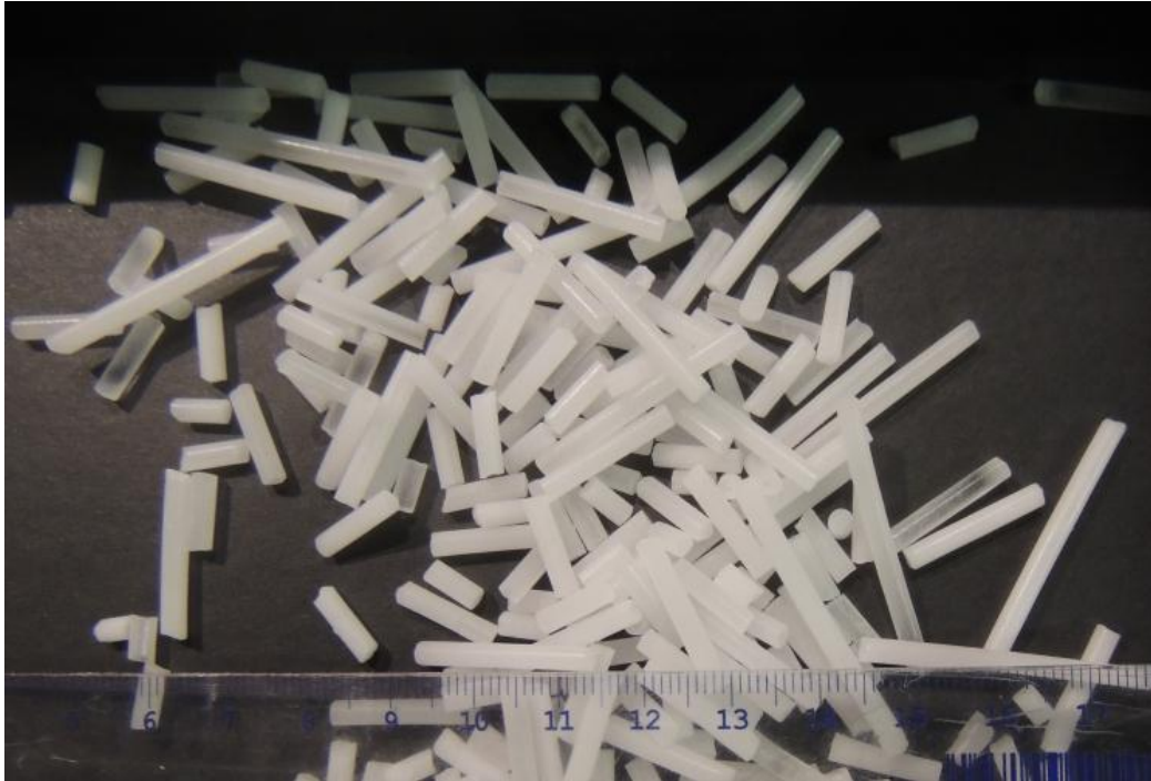
Figure 1: Fresh dry ice pellets (actual size)
