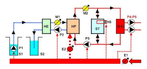
Figure 3: Depicted scheme of the connection of a heat pump water/water and electricity consumption
