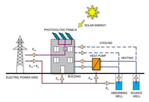
Figure 1: Schematic diagram of PV system, heat pump system and capillary mats
