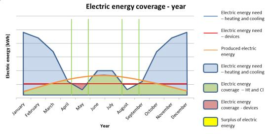
Figure 2: Electric power needs for heating, cooling, electricity and produced electricity by PV system during the year
