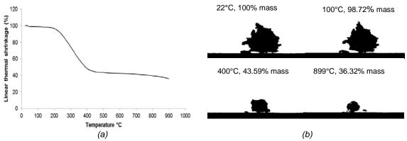
Figure 2: Linear thermal shrinkage curve (a) and images of mass degradation (b) for banana leaves briquettes.
