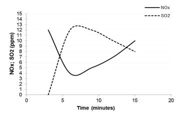
Figure 4: NOx and SO<sub>2</sub> levels relased during the briquettes combustion.
