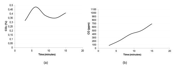
Figure 3: CO<sub>2</sub> (a) and CO (b) levels released during the briquettes combustion.
