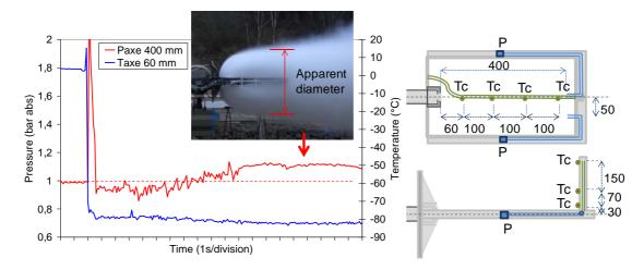
Figure 5: photograph and sketch of the dynamic pressure and temperature measurement in the expansion zone
