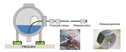
Figure 3: Drawing and photographs of the sphere, valves position and details of the release orifice
