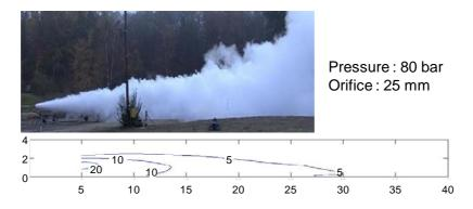
Figure 8: Example of mapping calculates from thermocouple field (picture and graph at the same scale).
