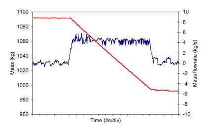
Figure 2: Example of mass lost from the sphere during a release (red curve) and instantaneous mass flowrate calculation (blue curve)
