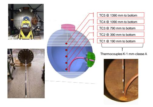
Figure 1: The 2 m<sup>3</sup> test reservoir and internal arrangement of the piping
