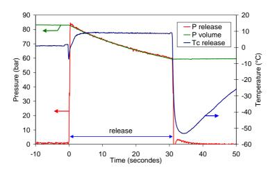
Figure 4: Example of temperature and pressure signals obtained at the orifice (12 mm orifice diameter)
