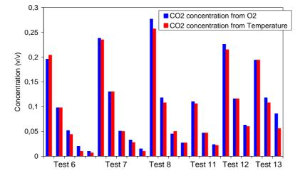
Figure 6: comparison between  $CO_2$  concentrations obtained via the temperature reading and the concentration deduced from the oxygen measurements for different tests
