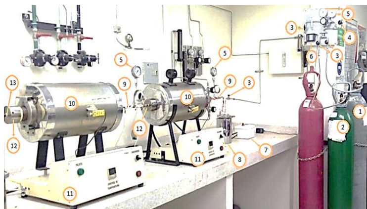
Figure 1: Experimental setup: 1) Cylinder with Ar, 2) Cylinder with CO 2 -O 2 -N 2 , 3) Flow valve, 4) Relief valve, 5) Pressure gauge, 6) Mass flow meter, 7) Humidifier temperature controller, 8) Humidifier, 9) Heating cord, 10) tubular electric furnace, 11) Furnace controller, 12) Reactor and coupons holder and 13) Gas and steam outlet
