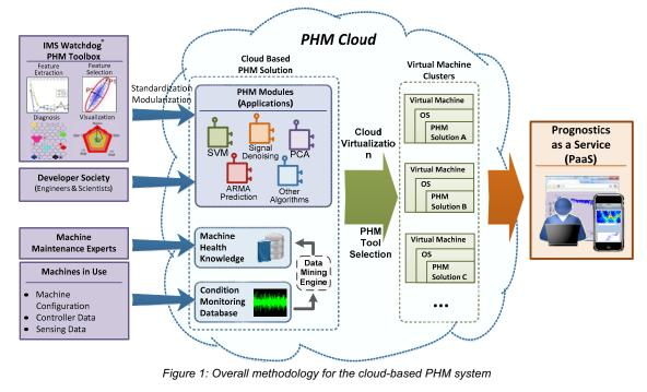
**PHM Cloud** 1. Prepare & customize PHM workflow Machine Info Machine configuration Type of data User requirement ata format PHM workflow configuration file Sample data Existing workflow template 2. Create virtual machine (PHM server) for current user Load preconfigured system Construct PHM image workflow based Initialize VM (including OS, support on configuration software, data transmission file module, WEB service, etc) 3. Output PHM results to WEB server
