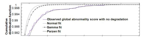
Figure 4: Observed and adjusted cumulative distribution function of ESC global abnormality score with no degradation.
