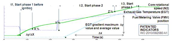
Figure 1: Engine start capability, ESC, indicators
