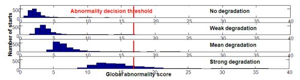
Figure 6: Prior abnormality decision threshold and global abnormality score distributions with three starter air valve degradation intensities.
