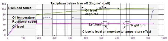
Figure 2: Engine oil consumption, EOC, oil level captures
