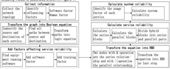
Figure 1 Process of network service reliability model
