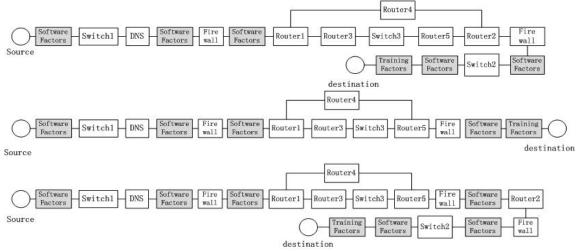
Figure 4 Reliability block diagram of three services
