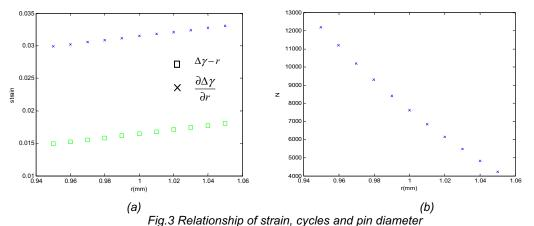
The strain and its sensitivity to pin diameter increase as pin diameter increase, so the fatigue life will decrease with the increase of pin diameter.
