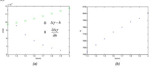
Fig.5 Relationship of strain cycles and solder joint height
