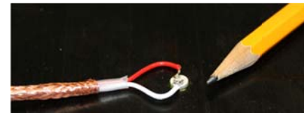
Figure 3: Detail of a surface mounted PZT transducer.
