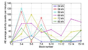
Figure 8: Acoustic Emission activity at different load levels
