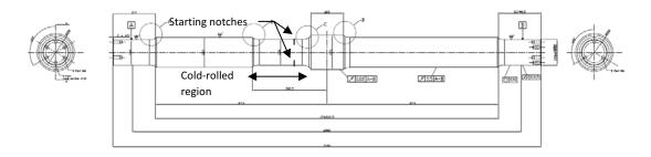
Figure 2: Drawing of the adopted full-scale specimen
