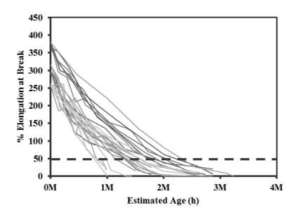
Figure 4: Normalized EAB data to a 50 °C Service Temperature
