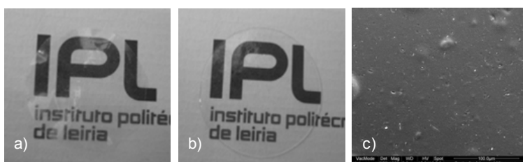
Figure 2: Macroscopic images showing the transparency of the crosslinked alginate film containing 25% of Aloe vera in dry (a) and wet state (b). SEM image of the surface of the crosslinked alginate film (c)
