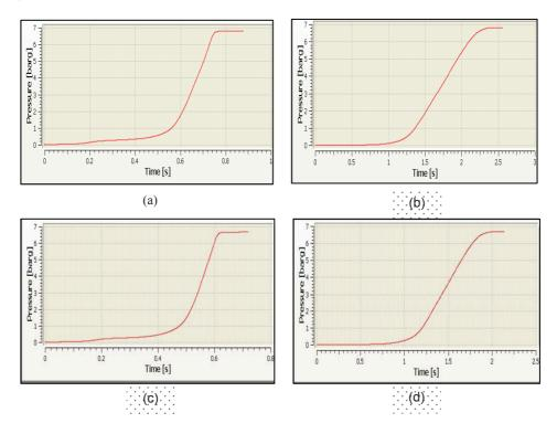
Figure 2: DESC simulation of polyamide 6.6 (dtex 1.7 and length 0.5 mm) explosions in (a) a 20-L spherical chamber and (b) a  $1-m^3$  spherical chamber; similarly for polyester (dtex 1.7 and length 0.5 mm) explosions in (c) a 20-L spherical chamber and (d) a  $1-m^3$  spherical chamber
