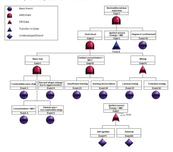
Figure 3: FTA diagram for nano-dust explosions
