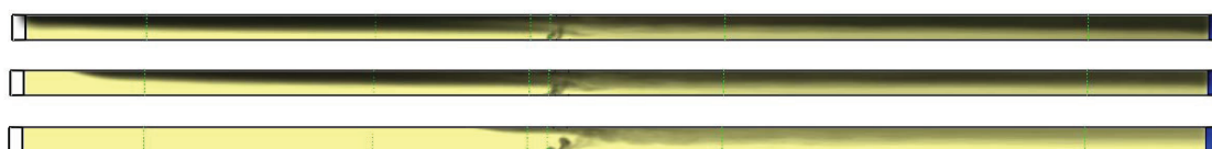
Figure 4: Estimated effect of the forced ventilation on the smoke backlayering for the Apte tunnel fire tests (from top to bottom, U=0.5 m/s, U=0.85 , and U=2.0 m/s).
