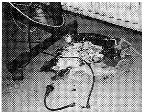
Figure 7: Wastepaper basket after smoldering fire showing damaged wires.
