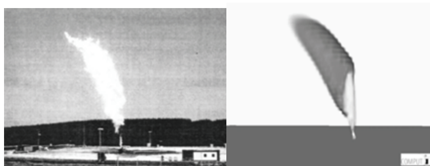
Figure 3: A 56 m flame from a high-pressure gas release experiment (left) vs. flame predicted by KFX ® (right)
