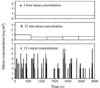
Figure 1: Time course of the odour concentration ( $ou_E / m^3$ ) for three time intervals. (a) one-hour mean value (e.g. output of a dispersion model), (b) 12-min and (c) 12-s mean odour concentrations observed at a single receptor point during a field study. The 12-s mean values were recorded and subsequently used to calculate 12-min and one-hour mean concentrations (source: Schauberger et al. (2012), modified from Nicell (2009)).
