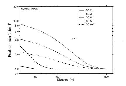
Figure 2: Distance depending peak-to-mean factor F for all stability class used by the AODM. The constant factor F = 4 applied by AUSTAL2000 is shown as a thin straight line (source: Piringer and Schauberger (2012)).
