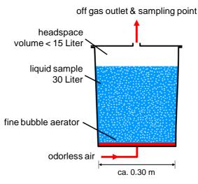
Figure 1: Sketch of the OEC test reactor
