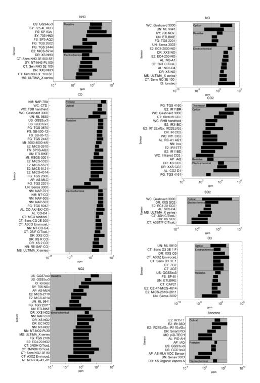
Figure 1: The concentration ranges of detection of the different sensors evaluated in the review. The dotted line represents the typical concentration of the European directives when available. The sensor that belongs to the same sensor technologies are grouped in the named grey areas.
