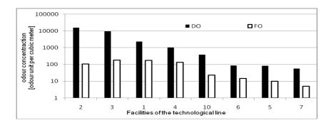
Figure 2: Ranking of the facilities (numbered according to the Figure 1) in terms of the odour concentrations
