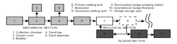
Figure 1: Wastewater treatment plant diagram
