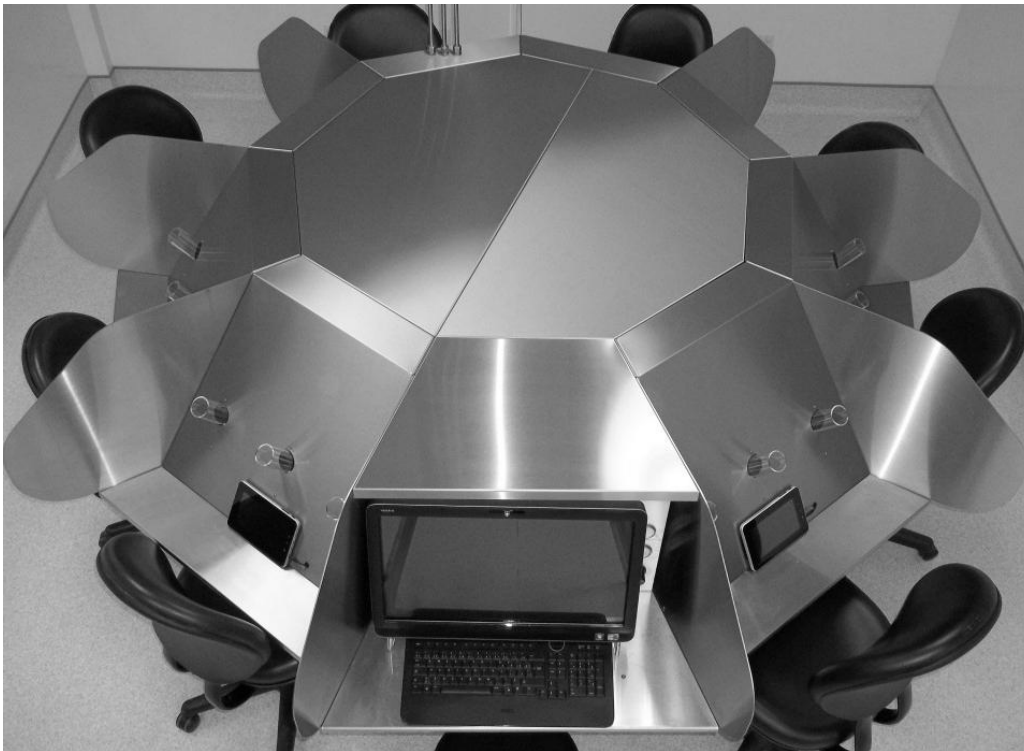
Figure 1: General design and structure of the 9-sided (nonagon) Onose-8 ® stationary dynamic dilution olfactometer operated at Consumaj laboratories in Canada.
