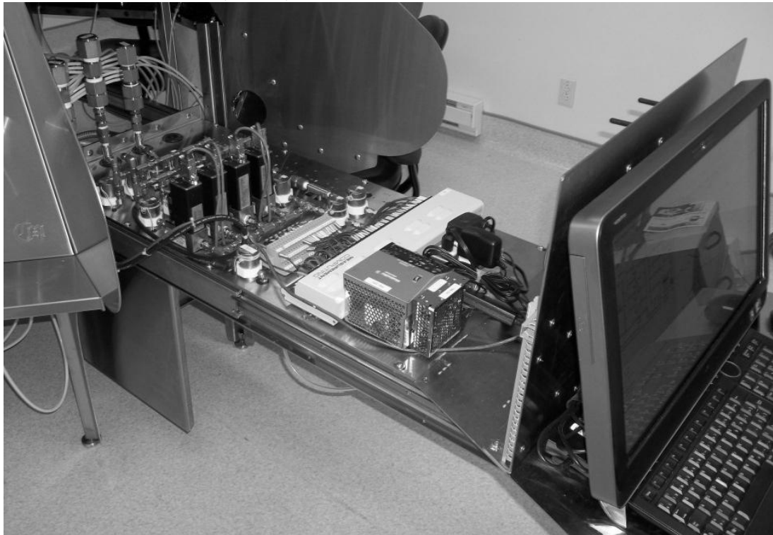
Figure 2: Presentation of the drawer supporting the main components of the fluidic circuit of the olfactometer. This drawer is located behind the operating station and can be pulled out from under the olfactometer's main structure.
