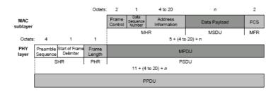
Figure 2: Data frame of IEEE 802..15.4/ZigBee Protocol.
