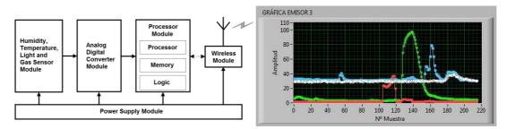
Figure 6: Block Diagram of the sensor nodes.
