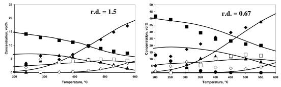
Figure 3: Experimental (points:  $\blacksquare$  H2O  $\diamond$ H<sub>2</sub>  $\blacktriangle$  CH<sub>4</sub>  $\square$  CO<sub>2</sub>  $\diamond$  CO  $\bullet$  C<sub>2</sub>H<sub>5</sub>OH) and equilibrium (lines) products distribution as a function of temperature for different catalysts in concentrated catalytic tests (Total flow rate=1000 Ncc/min; GHSV=15,000 h-1; r.a.=3)
