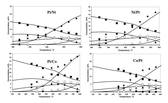
Figure 2: Experimental (points:  $\blacksquare$  H2O  $\bullet$ H2  $\blacktriangle$  H4  $\square$  CO2  $\diamond$  CO  $\bullet$  C2H5OH) and equilibrium (lines) products distribution as a function of temperature for different catalysts in concentrated catalytic tests (Total flow rate=1000 Ncc/min; GHSV=15,000 h-1; r.d.=4; r.a.=3)
