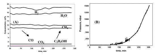
Figure 4: Experimental product distribution (A) and pressure drops profile (B) as a function of time during the stability test in concentrated catalytic tests for Pt/Ni catalyst (Total flow rate = 1000 Ncc/min; GHSV = 15,000  $h^{-1}$ ; r.d.= 4; r.a.=3)
