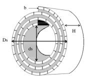
Figure 1. Main geometrical variables of a spiral heat exchanger
