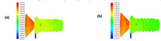
Figure 2: (a) contours of static temperature of reactor walls for  $m_p = 0.2$  g/min, (b) contours of static temperature of reactor walls for  $m_p = 0.6$  g/min
