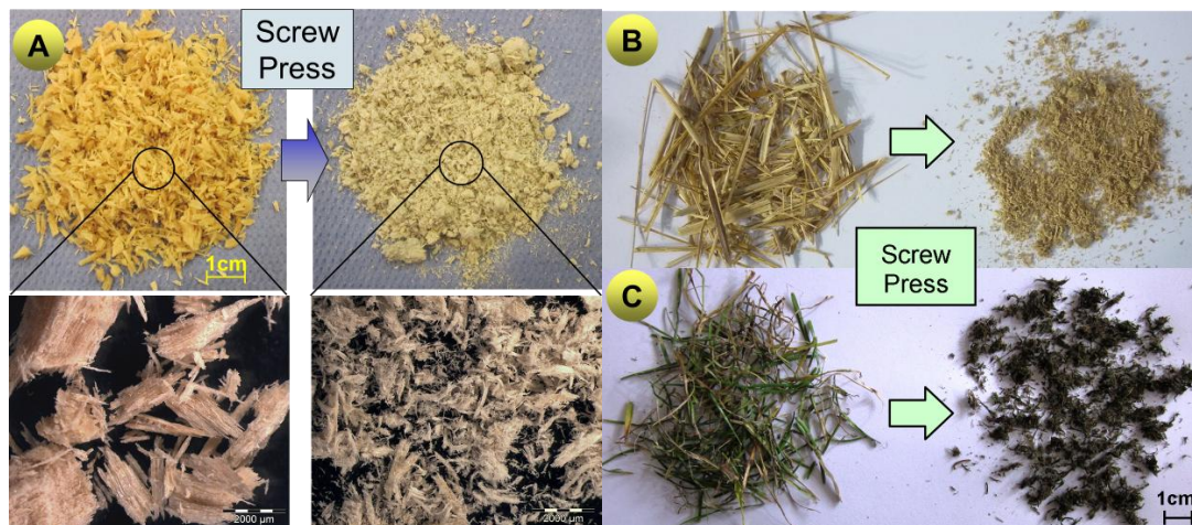
Figure 2: Mechanical pretreatment of beech wood (A), reed (B) and ryegrass (C) using a screw press
