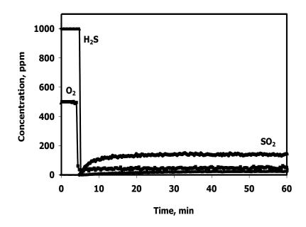
Figure 4: Stability test of  $V_2O_5$ /CeO<sub>2</sub> at T=250 °C (1000 ppm H<sub>2</sub>S, O<sub>2</sub>/H<sub>2</sub>S=0.5).
