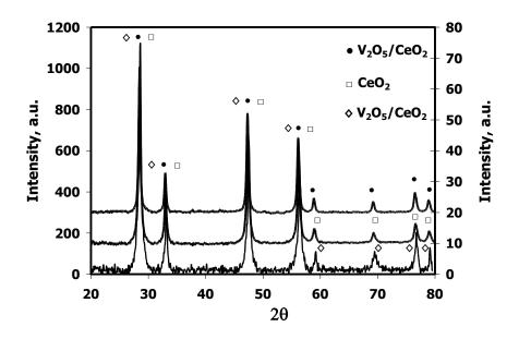
Figure 1: X-Ray diffraction patterns of CeO<sub>2</sub> and of the catalyst V<sub>2</sub>O<sub>5</sub>/CeO<sub>2</sub> before (•) and after the catalytic test ( $\Diamond$ ).
