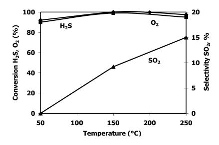
Figure 3: Conversion of H<sub>2</sub>S, O<sub>2</sub> and SO<sub>2</sub> selectivity in the range T=50-250 °C
