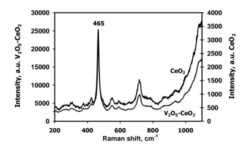
Figure 2: Raman spectra of CeO<sub>2</sub> and of the catalyst V<sub>2</sub>O<sub>5</sub>/CeO<sub>2</sub> before of the catalytic test.
