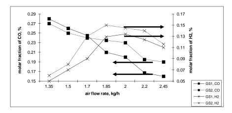
Figure 4. Molar fraction of hydrogen and carbon monoxide against the air flow rate
