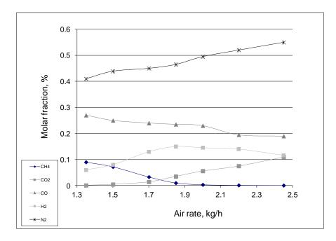
Figure 3. Molar fraction of hydrogen and carbon monoxide against the air flow rate
