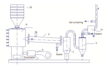
Figure 2. Schematic diagram of the experimental system
