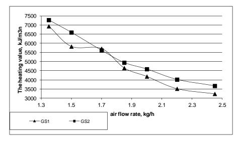
Figure 6. The heating value of syngas against the air flow rate
