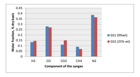
Figure 5. Comparison of the syngas composition in the case of dry and wet sewage sludge feedstock
