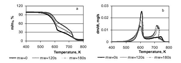
Figure 3: Temperature dependence of the mass loss (a) and rates of the mass loss (b) of untreated and pre-treated wood biomass combustion from the TG analysis.
