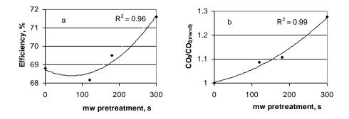
Figure 5: Effect of the microwave pre-treatment duration on the variations of combustion efficiency (a) and  $CO_2$  volume fraction (b).
