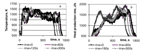
Figure 4: Effect of the microwave pre-treatment duration on the time-dependent variations of temperature (a) and heat production rates (b) at different stages of thermo-chemical conversion.
