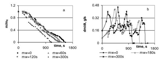
Figure 2: Effect of the microwave pre-treatment duration on the relative mass loss (a) and mass loss rate variations (b) of pre-treated samples at different stages of thermo-chemical conversion.
