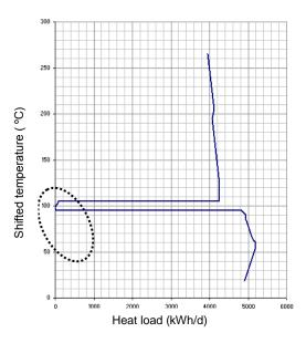
Figure 4: GCC of Scenario 3, incorporating solar energy, the economizer and the heat pump
