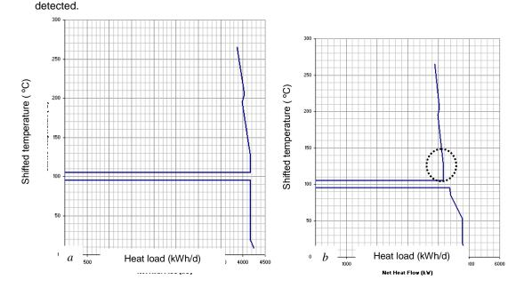
Figure 2: GCC of Scenarios before incorporating thermosolar energy; a. Scenario 1, and b. Scenario 2
