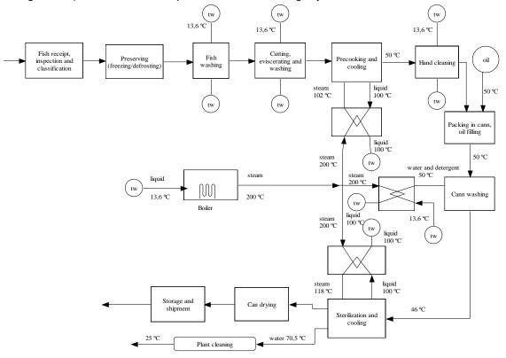
Figure 1. Scheme of the canning facility (tw: tap water)
