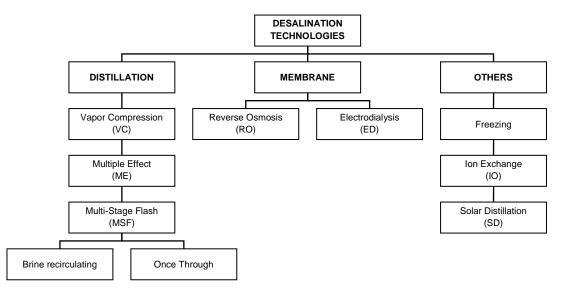
Figure 1: Classification of desalinating processes
