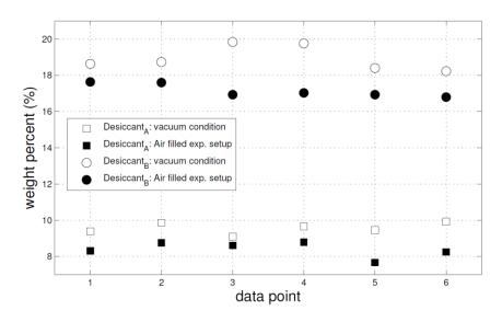
Figure 2: Comparison of the storage capacity in weight percent of desiccant A and desiccant B at 230 °C and with a generated vacuum or air filled in the experimental setup
