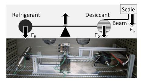
Figure 3: Picture and schematics of the test setup to investigate the sorption velocity and capacity for different material combinations.
