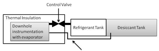
Tube for gaseous refrigerant to the Desiccant
