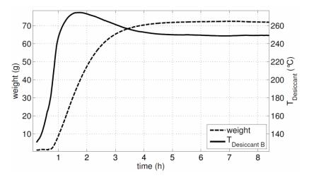
Figure 4: Weight of stored refrigerant and temperature of desiccant B with vacuum condition in the experimental system.
