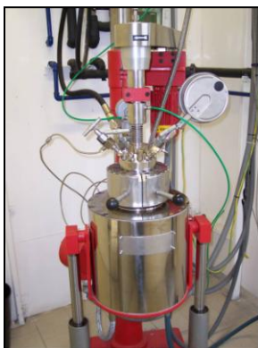
Figure 1: Wet Oxidation reactor used in the experimentation.
