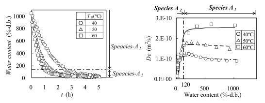
Figure 1: Dehydration response curves as a function of the drying temperatures (RH = 20 %).
