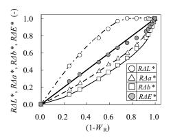
Figure 4 Color parameters as a function of the ratio of dehydrated water  $T_D=40^{\circ}C,RH=20\%$ )
