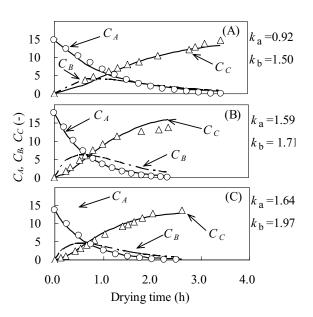
Figure 6: Fitting of the computer simulation response curves to the experimental data based on the consecutive reaction model ( $T_D = (A)$  40 °C, (B) 50 °C, (C) 60 °C), RH=20 %.
