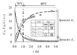
Figure 9: The two step dehydration response curves. RH=20 %
