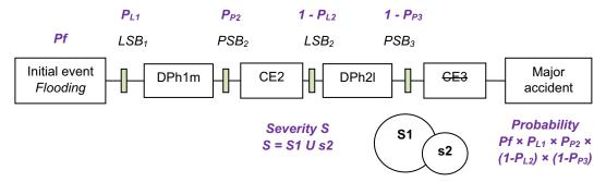
Figure 6: Probability and severity assessment - Example of calculation with safety barriers
