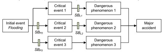
Figure 3: Representation of accidental sequences causing by flooding
