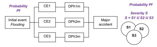
Figure 5: Probability and severity assessment - Conservative calculation
