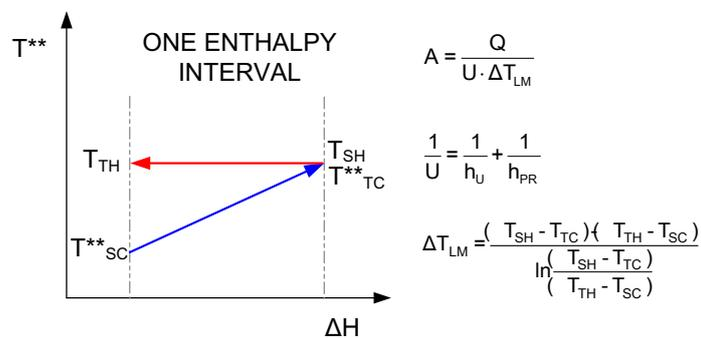
Figure 4: Determining the heat transfer area in one EI
