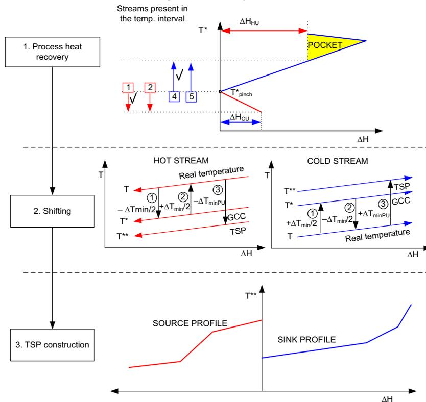
Figure 2: Constructing TSPs
