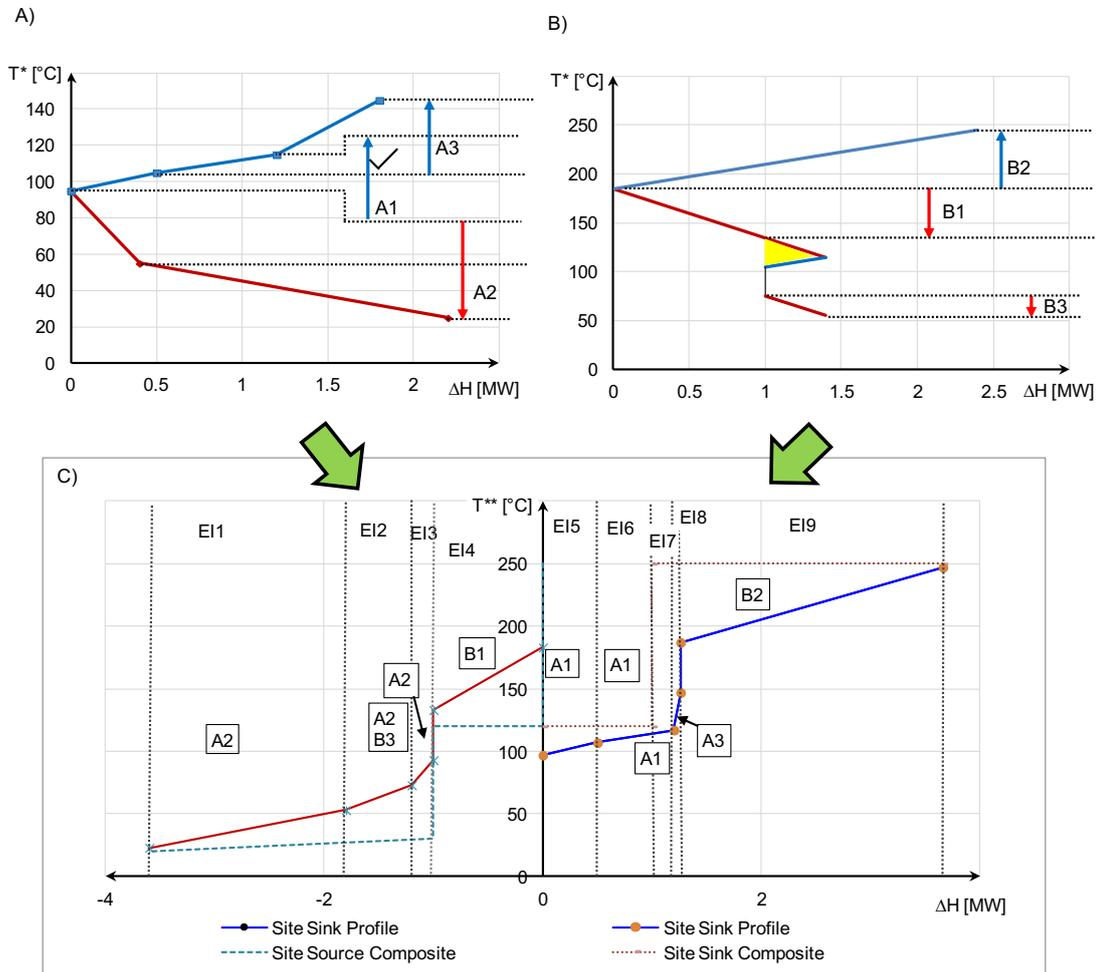
Figure 5: GCC of A) Process A and B) Process B and the c) TSPs
