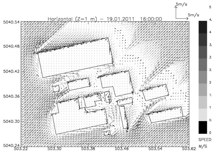
Figure 1. Wind field at 1 m height in D5 atmospheric conditions.
