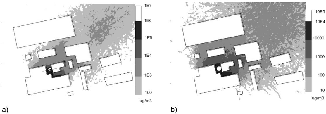
Figure 2. SO<sub>2</sub> average concentration after 600 s of accident in stability conditions F2 (a) and D5 (b).
