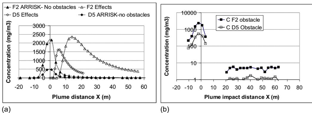
Figure 4. Ground Plume impact along the direction of plume dispersion for different models and meteorological conditions: no obstacle (a) and obstacle (b) simulations.
