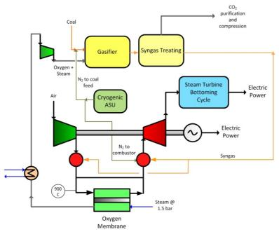
Figure 3: Process block diagram for OTM integrated IGCC plant with CO<sub>2</sub> capture
