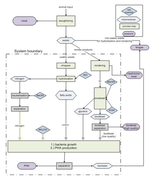
Figure 1: Process flowchart
