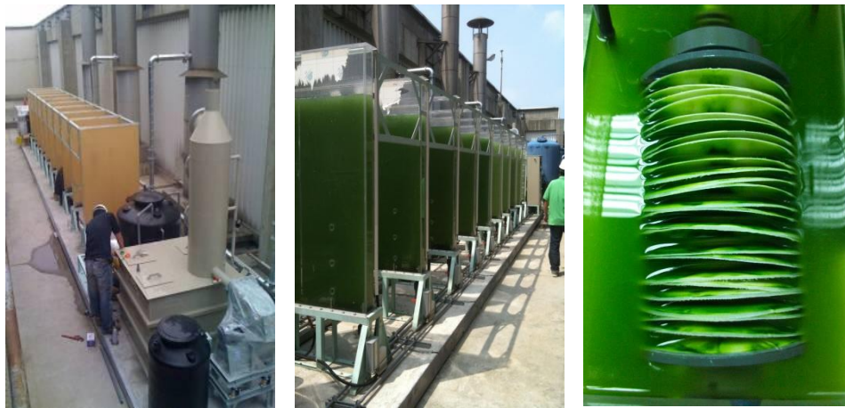
Figure 4: Pilot-scale integrated system: (a) site layout showing the scrubber, and a series photobioreactors; (b) photobioreactors in operation with microalgae; (c) membrane harvesting.
