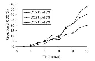
Figure 2:. Reduction of CO<sub>2</sub> at various CO<sub>2</sub> input concentration constant light intensity of 360 lumen
