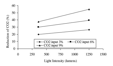
Figure 5: The effect of light intensity on CO<sub>2</sub> reduction
