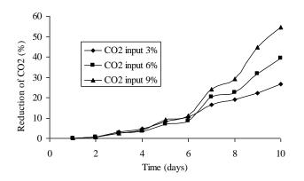
Figure 3: Reduction of  $CO_2$  at various  $CO_2$  input concentration with constant light intensity of 1250 lumen
