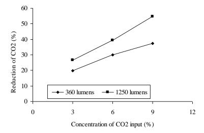
Figure 4. The effect of CO<sub>2</sub> input on CO<sub>2</sub> reduction
