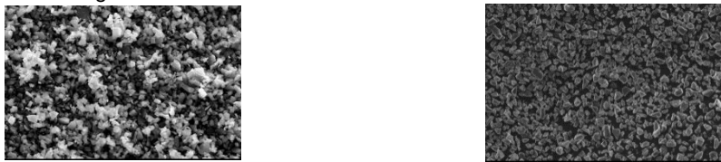
(a) Powder after the dry ball milling for 15 hours (b) Powder after the wet ball milling for 10 hours
