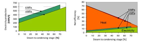
Figure 2:Specific electricity production
