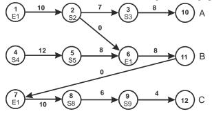
Figure 3. S-graph representation of task sequence 1-6-7 for equipment unit E1 with NIS policy.
