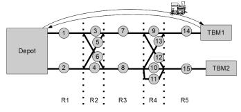
Figure 4. Railway network of the supply train routing problem.
