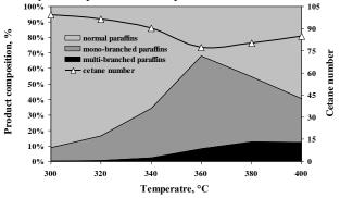
Figure 8: The composition and the estimated cetane number of the products in function of the temperature (LSHV = 1,0  $h^{-1}$ , p = 40 bar,  $H_2/HC$  ratio = 400 Nm<sup>3</sup>/m<sup>3</sup>)
