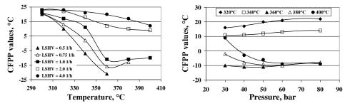
Figure 6: The CFPP values of the productsFigure 7:in function of the temperature  $(p = 40 \text{ bar}, products in H_2/HC ratio = 400 \text{ Nm}^3/\text{m}^3)$ (LSHV=1.0)
