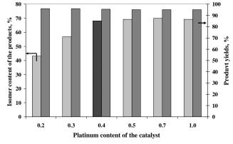
Figure 1: The yield and the isomer content of the target products in the function of platinum content of the catalysts ( $T = 360^{\circ}C$ , p = 40 bar,  $H_2/HC$  ratio=  $400 \text{ Nm}^3/\text{m}^3$ )
