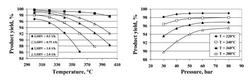
Figure 2: The yields of products in function of the temperature (p = 40 bar,  $H_2/HC$  ratio  $= 400 \text{ Nm}^3/\text{m}^3$ )
