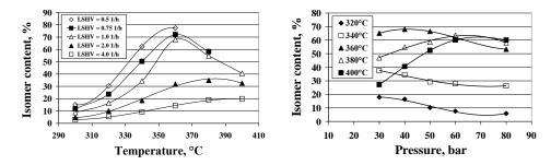
Figure 4: The total isomer content of the Figure 5: The total isomer content of the product in function of the temperature (p = product in function of the pressure  $40 \text{ bar}, H_2/\text{HC} \text{ ration} = 400 \text{ Nm}^3/\text{m}^3$ ) (LSHV=1.0h<sup>-1</sup>,  $H_2/\text{HC} \text{ ratio} = 400 \text{ Nm}^3/\text{m}^3$ )
