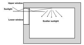
Figure 4: Illumination principle of lighting clapboard
