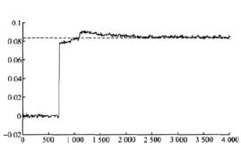
Figure 6: The temperature rising velocity tracking curve(only the first 15 000 s are shown)in the heating experiment of the furnace with Te= 400 s
