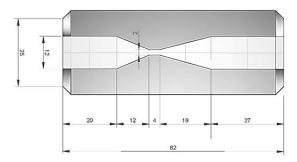
Figure 3: Sketch of the Venturi tube
